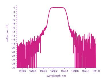
parameters (strength, FWHM, SLSR). Apodized FBGs are useful in sensing applications, signal and Brillouin scatter filtering and others. Possible value of SLSR for different grating strength is -10dB to -30dB. The reflection spectrum of Apodized HR FBGs is presented in the graph.
